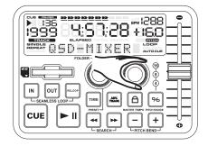
**Figure 3:** Turning the track knob clockwise will take you to the to the next track.
